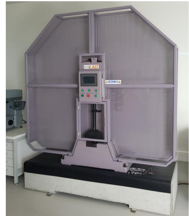
Impact toughness testing using the Charpy method
