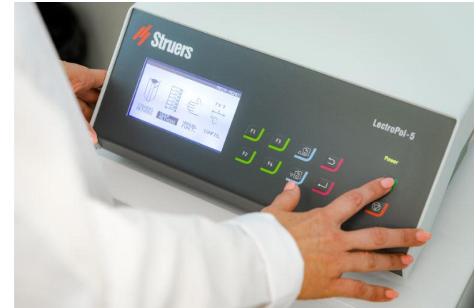
Device for electrolytic polishing and etching of materials
