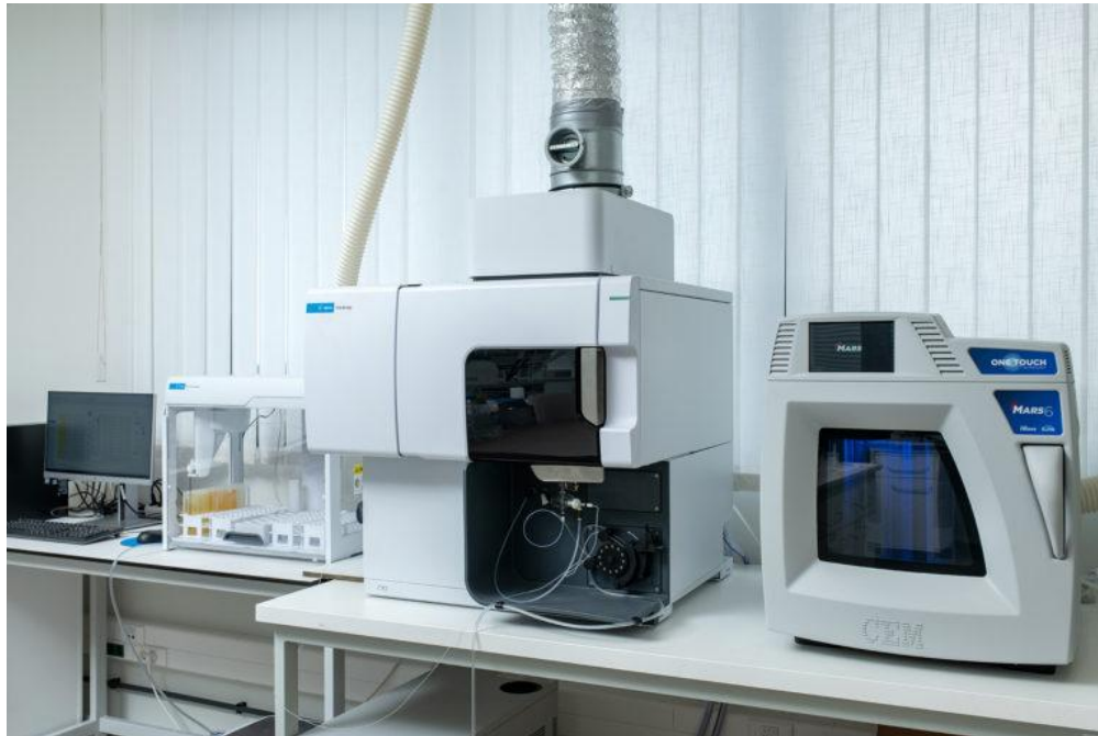
Inductively Coupled Plasma Optical Emission Spectrometer (ICP-OES)
