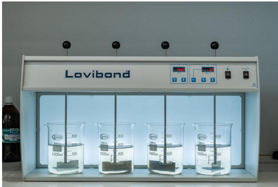
Jar tester – simulating processes at a water treatment plant.
