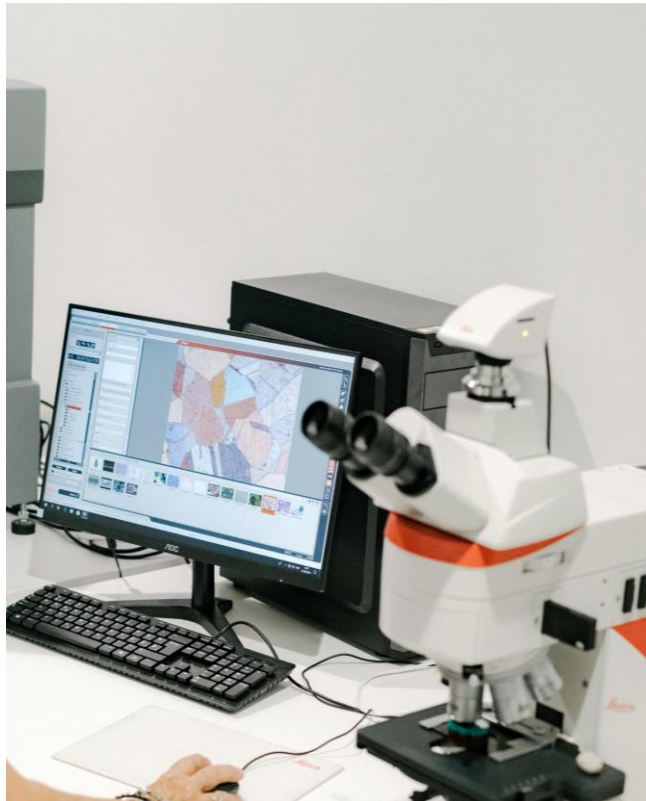
Metallographic testing – Leica DM4 microscope with magnification up to 2000x
