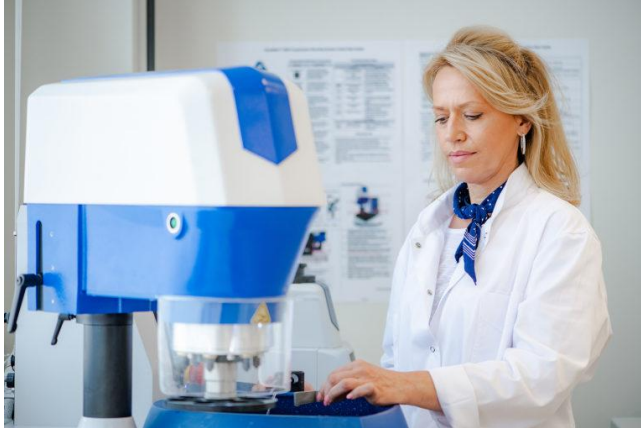
Semi-automated devices for precise grinding and polishing of metals
